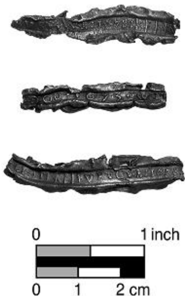
Figure 3. Conserved window leads at HSMC sometimes show maker's marks and dates.
